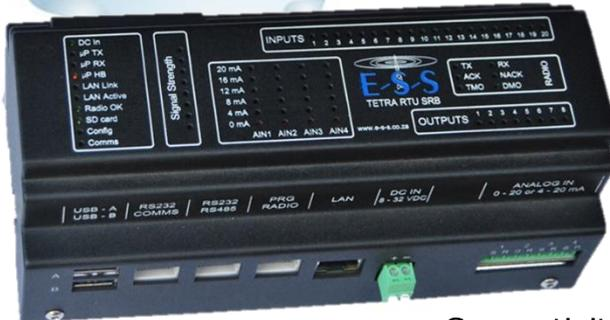
Various remote analog and digital sensors can be used with a choice of different communication technologies. The ESS TETRA-RTU allows for exceptional flexibility and modularity with the ability to provide 100% redundancy for critical management.
